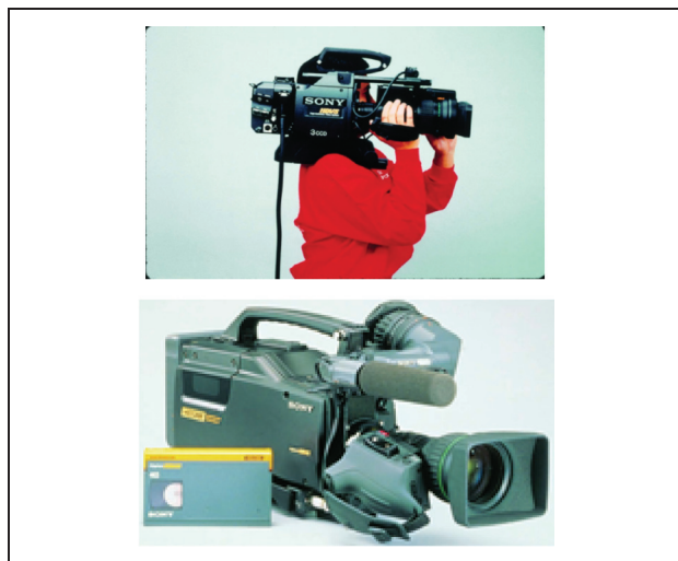
FIGURE 15. (Top) First CCD HDTV camera HDC-500 based on a 1 in. image format size from Sony; (Bottom) only five years later, the world's first integrated 2/3 in. HDTV camcorder HDW-700.
