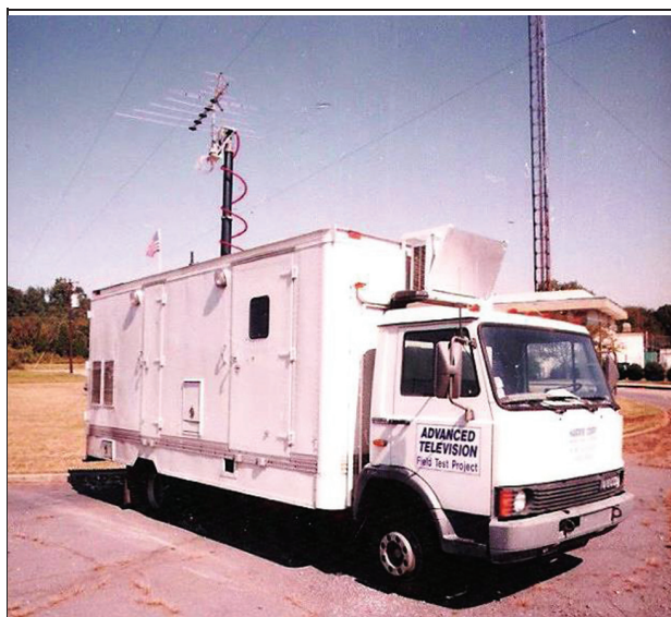
FIGURE 13. Vehicle used for measurements in connection with HDTV field test operations in Charlotte, North Carolina.
