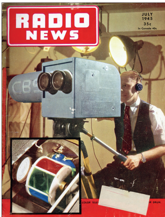
FIGURE 1. This July 1945 edition of Radio News described a color TV scanning system using a spinning, synchronized color wheel.
