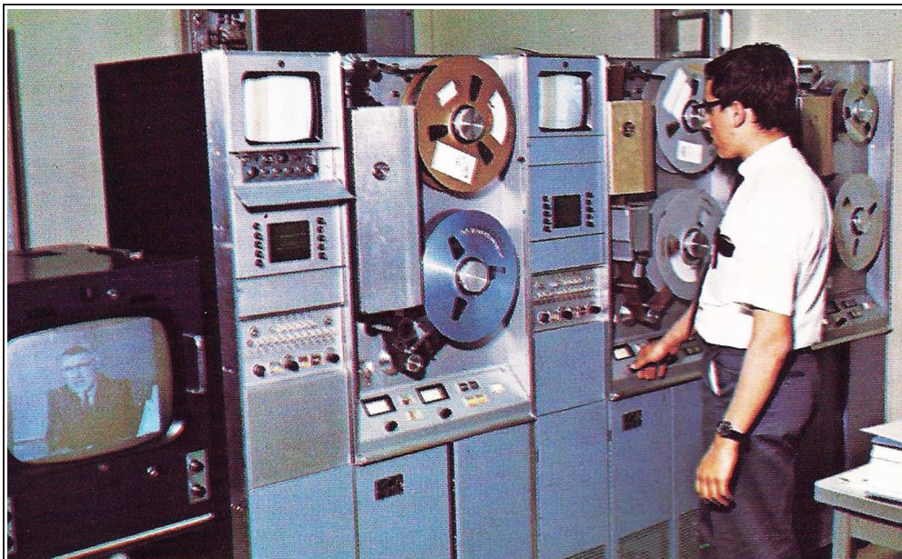
FIGURE 15. The 1956 2 in. “quad” videotape format was still in use in the mid-1970s, but this would eventually be replaced by smaller and more economical to operate 1 in. “type C” VTRs. The machines shown here are from RCA.
