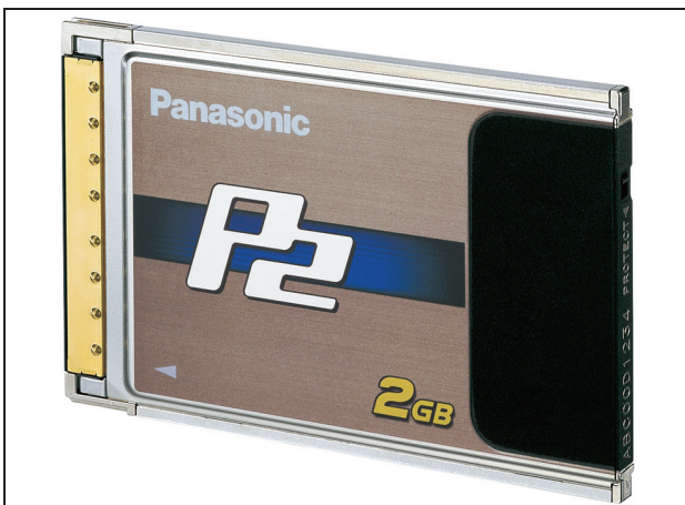
FIGURE 20. Panasonic's first-generation P2 solid-state digital video storage card has a 2-Gbyte capacity.
