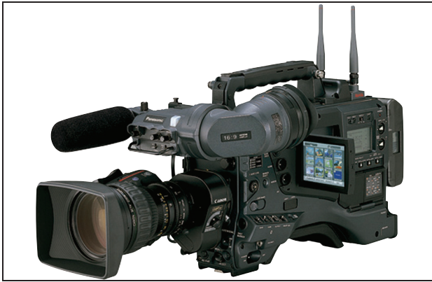
FIGURE 19. This 2004 Panasonic camcorder marked the beginning of video capture in the field in solid-state storage media (P2 card) and also helped to define TV's tapeless production workflow.
