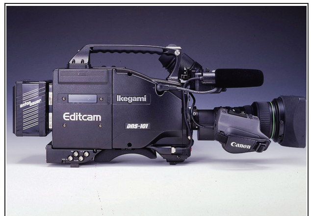
FIGURE 18. The Ikegami “Editcam” (an Ikegami and Avid joint venture) featured a dockable disk drive for speeding up editing operations. The 1995 camcorder was an early entrant in the “tapeless” TV production workflow.
