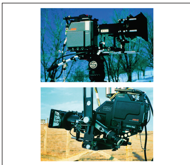
FIGURE 14. In 1984, Sony introduced the HDC-100—the world's first commercially available HDTV camera (shown on the left with Nikon lens), and by 1987, a second-generation camera saw collaboration between Sony and Panavision on an HD electronic cinematography camera.
