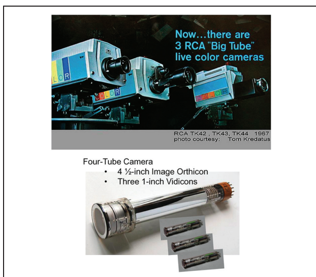
FIGURE 9. Four-tube cameras developed by RCA in the 1960s, with the camera on the right featuring a novel new image isocon (1967), which unfortunately fell victim to the meteoric rise of the Plumbicon.
