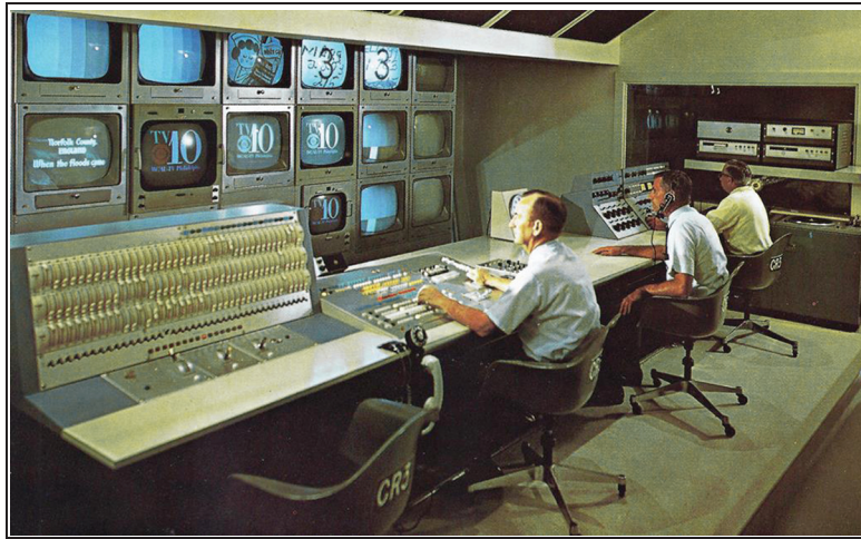
FIGURE 4. A typical studio control room in the 1970s. (The studio lighting control console is on the left, the production switcher in the middle, and the audio mixer on the right.)
