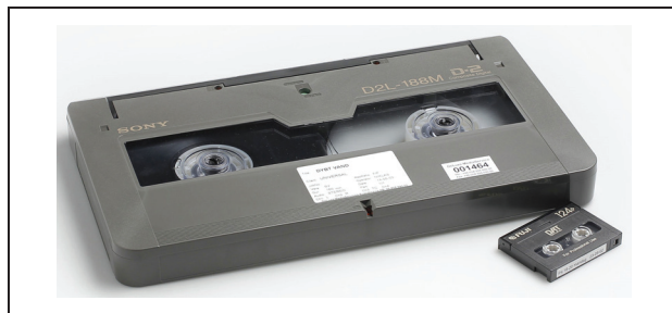
FIGURE 11. D2 digital tape cassette (left) next to a digital audio tape (foreground, right) for scale. iii
