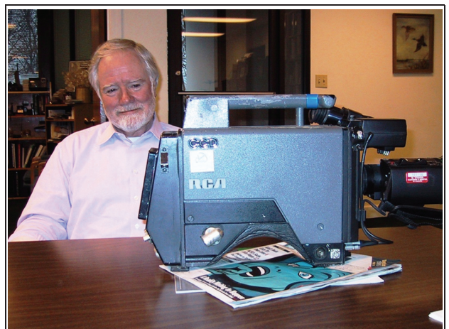
FIGURE 7. Larry Thorpe with the first "chip" imager broadcast TV camera, RCA's CCD-1. It was first shown at the 1983 SMPTE conference.
