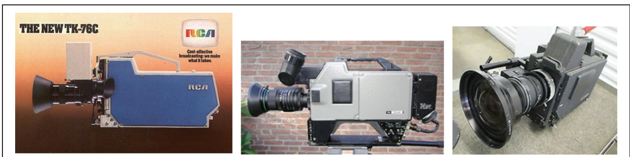
FIGURE 12. Evolution in 2/3 in. image format cameras—the pioneering RCA TK-76 on the left, which was soon challenged by the Ikegami HL-79A on the center—and Ikegami's later foray into electronic cinematography with their EC-35 (Right).
