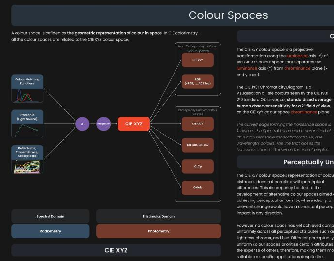
Spectral radiant energy is converted into CIE XYZ tristimulus values, *i.e.*, three dimensional geometric representation, by integrating the result of the product of the reflectance, transmittance or absorptance spectral distribution of a sample and the spectral distribution of a light source (or illuminant) with the colour matching functions, i.e., linear combination of the cone cells sensitivities
